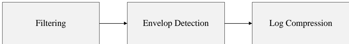
Figure 3-18: Mid – End unit of a typical Ultrasound system
